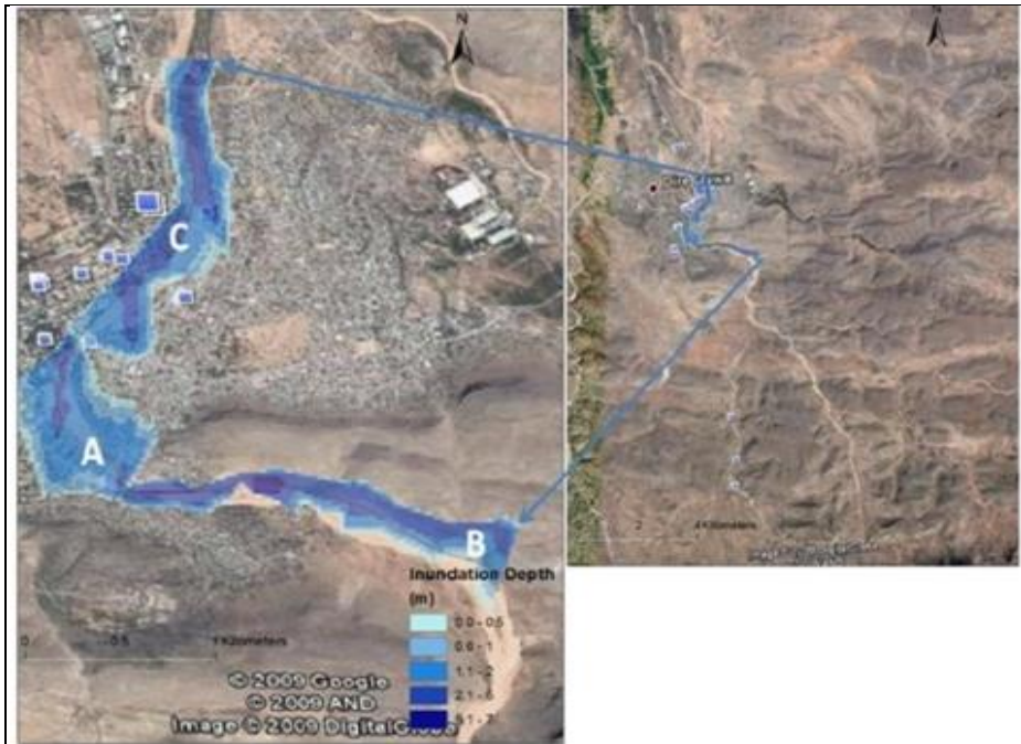
Figure 3.9: Inundation map of Dechatu catchment. The symbol in the map shows the location of residential areas inundated and cut-off road in the 2006 flooding.
