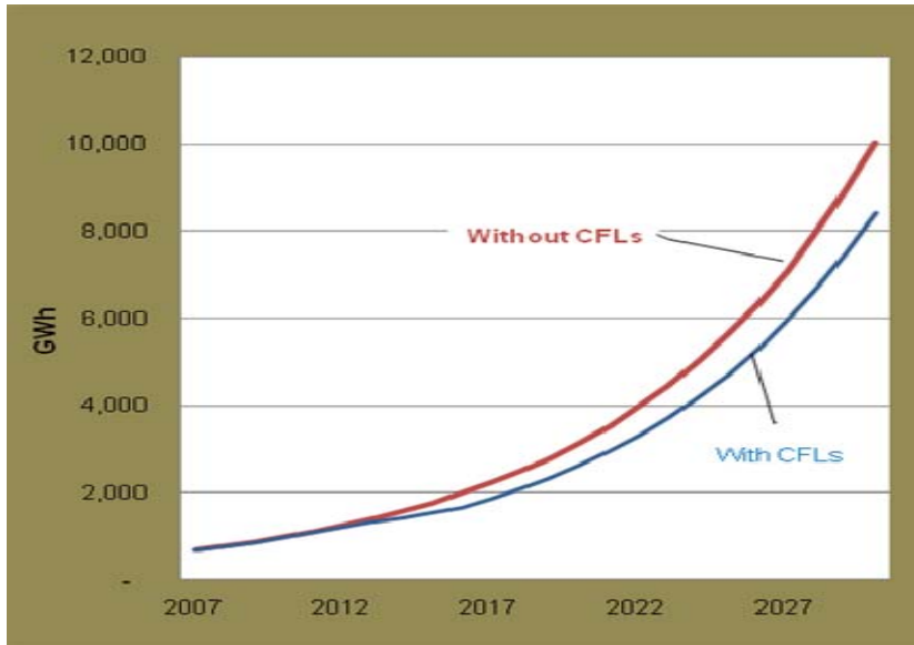
Figure 10.18: Services sector power demand with and without phasing-out of incandescent light bulbs
